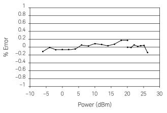
Typical E9300B/01B power linearity at 25 °C, after zero and calibration, with associated measurement uncertainty.
