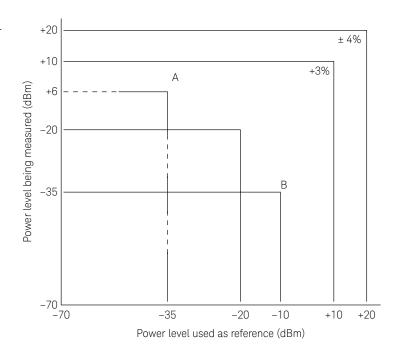
Figure 1. Relative mode power measurement linearity with EPM Series power meter/E-Series CW power sensor at 25 °C  $\pm$  5 °C (typical).
